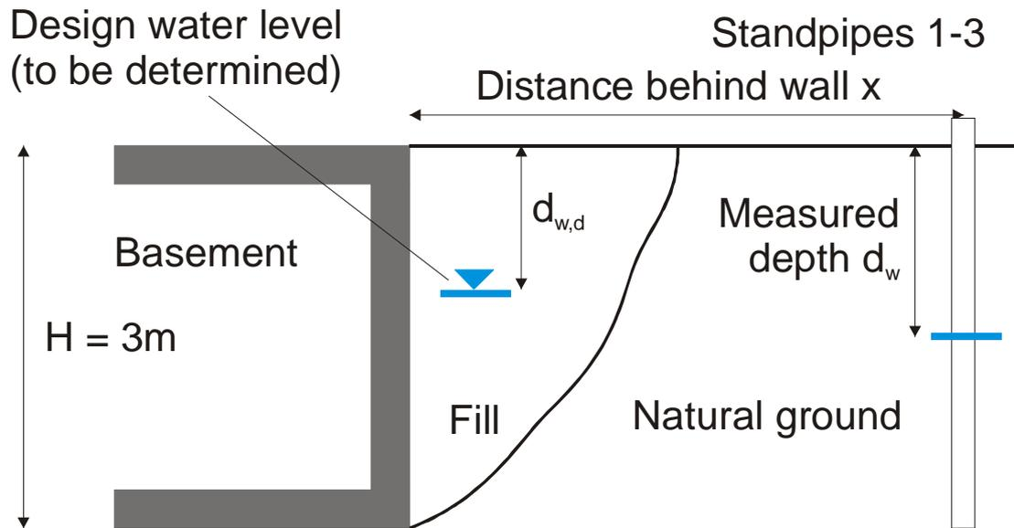
This example is designed to compare engineers' assumptions about water pressures acting on the face of a basement wall. The wall will NOT be provided with a drainage system. Ground surface behind the wall is horizontal will be paved in the long term.
